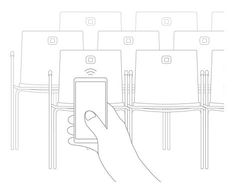
**Several components, one solution.** In addition to the displays on the chairs, the interactive seat numbering requires a server with the system software, access points for data transmission, and a handheld scanner for localising the chairs.
